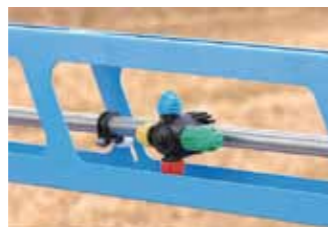
Folded metal frame with integrated spray circuit, nozzle holder and nozzles.
