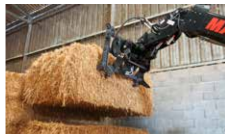
Bale spike For handling round & square bales – 2 teeth, 130 cm Ø 40 mm - 90 cm between centres.
