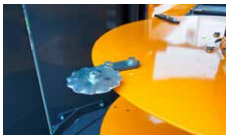
Cutting knives on the straw-bedding disc Passage of long or tacky bales and round bales.
