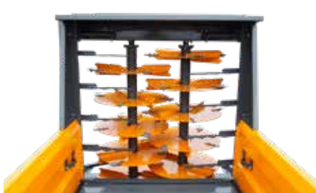
2 Rotor heights To adapt the machine according to the square bales used.
