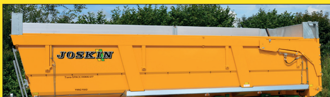
Combination of alu extensions and a hydraulic steel extension (50 cm)
