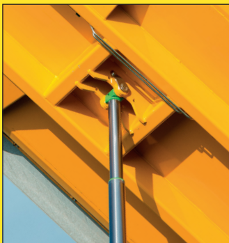
Anchoring point of the ram on the body
