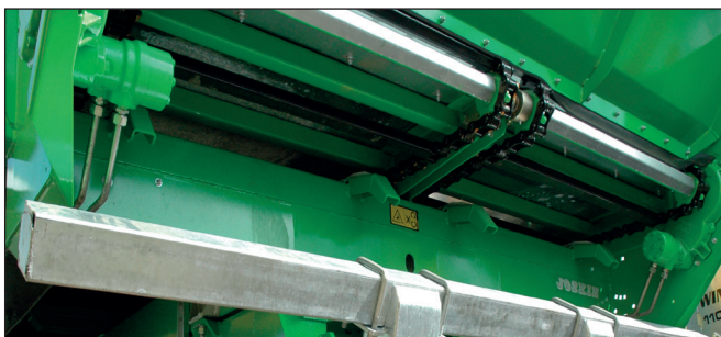
Moving floor driven by two hydraulic motors
