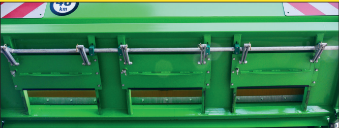
Two extra grain chutes as an option
