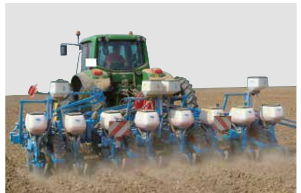
8-row folding planter (inter row spacings of 80cm)
