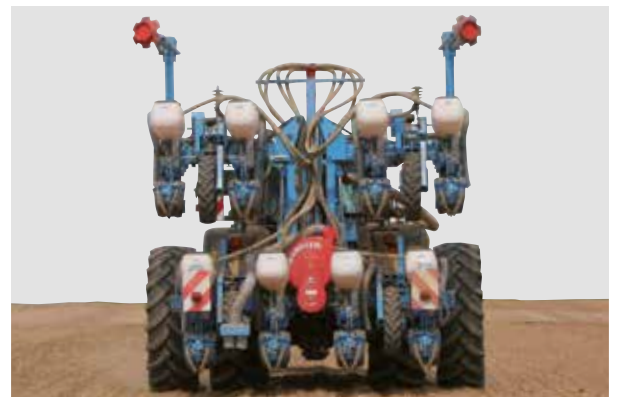
8-row folding planter in transport position
