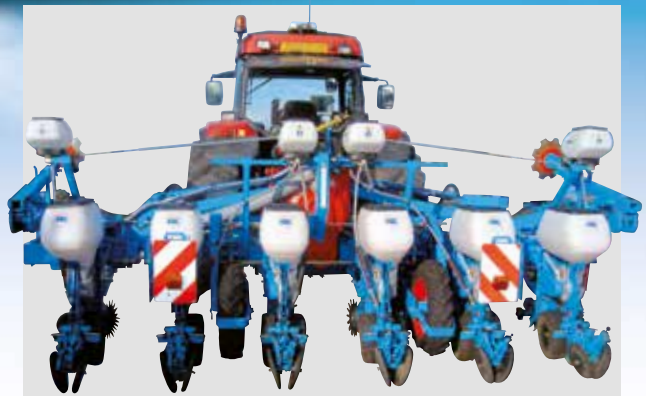
6-row folding planter (inter row spacings of 75cm)
