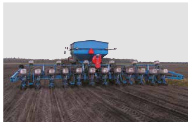
12-row folding planter (inter row spacings of 75cm)
