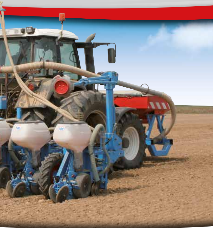
6-row folding planter (inter row spacings of 75cm)
