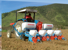
Multi-purpose pneumatic planter with NC shoes
