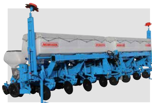
8-row planter with fertilizer (75cm inter row spacings)
