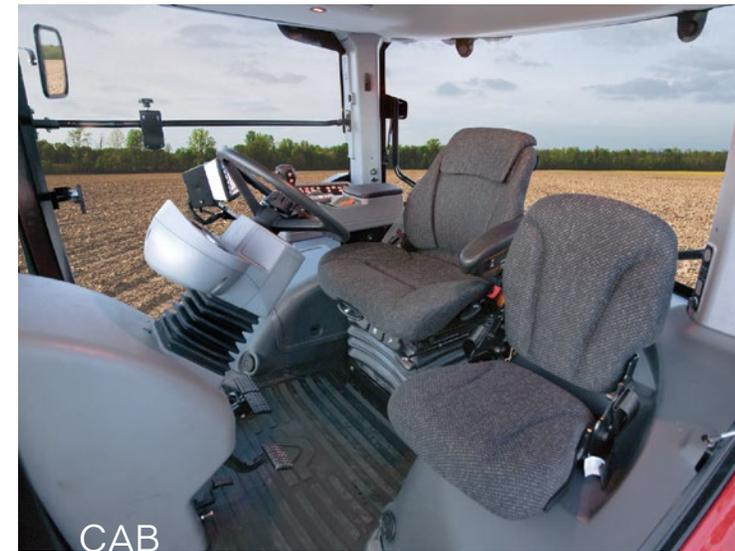
The new Versatile MFWD tractors offer the largest cab in its class. The cab interior is 26% larger than previous models with a total volume of 149 cu. ft. (4.22 cu. m). The total area of usable window glass is 73.5 sq. ft. (6.83 sq. m) offering an expansive view. The new cab and hood design also increase forward visibility over the previous generation of Versatile MFWD tractors. New eyeball air vents and floor venting have been added to increase operator comfort and reduce window fogging.
